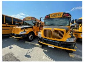
The District took delivery of its two Type C electric buses in July 2022. These buses are manufactured by International and distributed by Western Canada bus. Replacing our 85-seat Type D diesel buses, these 72 seat electric buses have an estimated range of 230 km.
