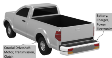
Figure 7: Blue Dot Motorworks Narwhal Retrofit Plug-In Hybrid System
